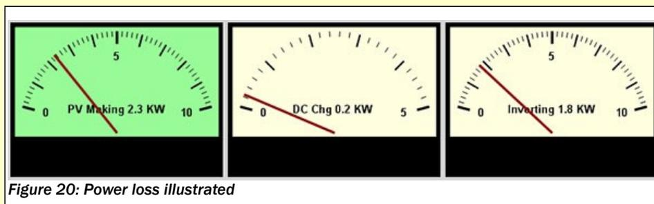
not convert 100% of DC power to house current, so some is lost there, too. It is difficult to predict how efficient a system will be, unless the manufacturer specifies it.
