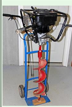
**Figure 45: Power earth auger stored on a hand truck for easy transport.**
