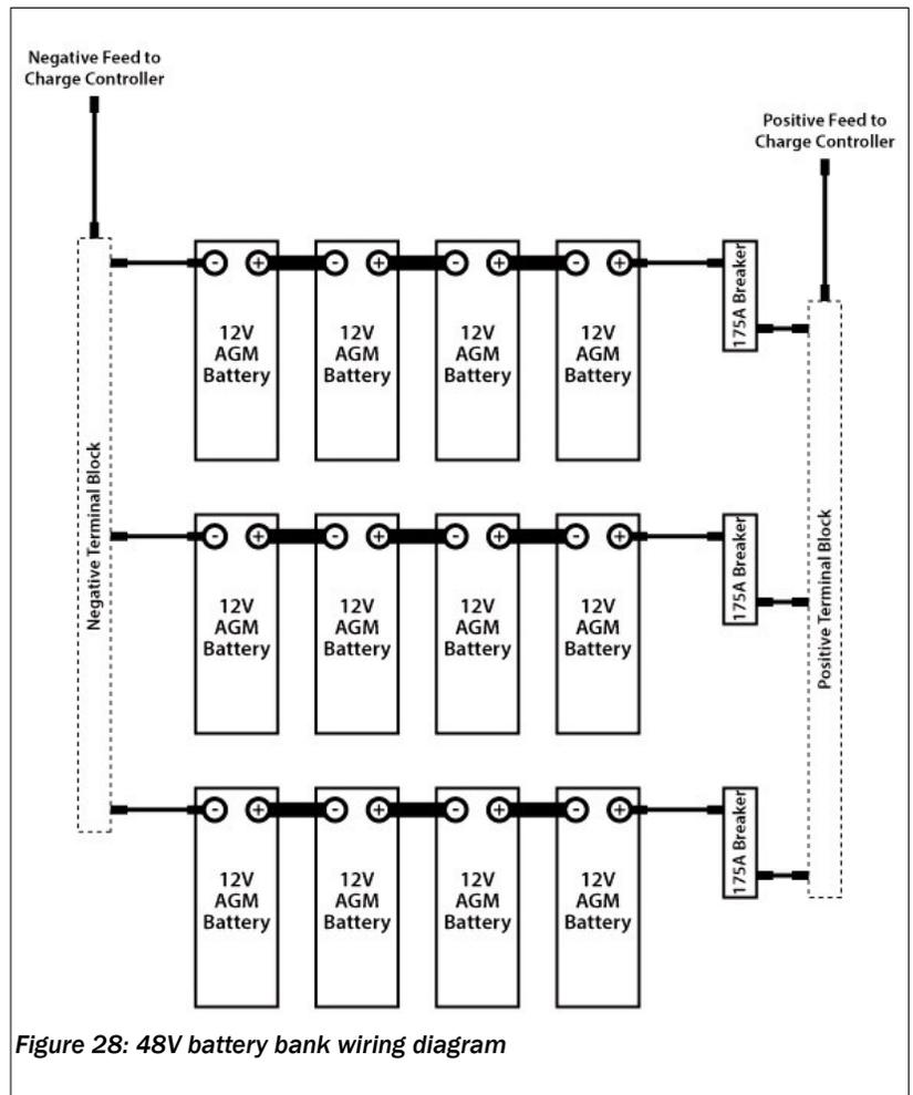
Figure 28: 48V battery bank wiring diagram
