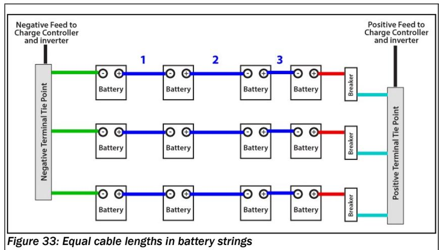
Figure 33: Equal cable lengths in battery strings
