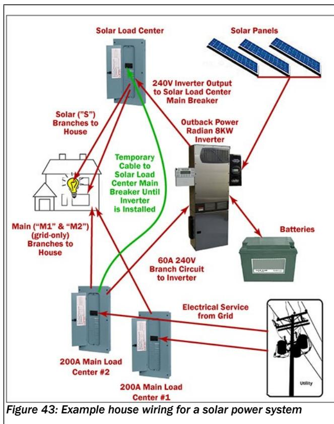
Figure 43: Example house wiring for a solar power system
