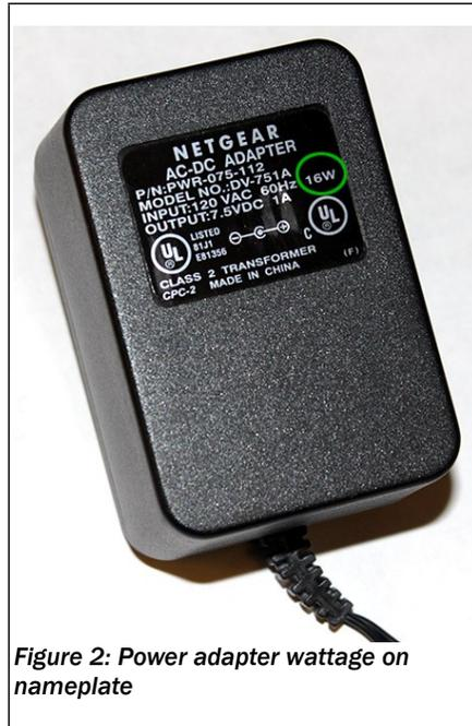
Figure 2: Power adapter wattage on nameplate
